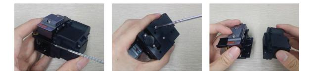
iii. Open the cover; with the slider advanced, then unscrew the set screw using a wrench as in the figure.
