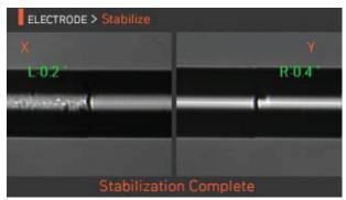
i. After stabilizing the electrodes, the arc calibration should be conducted again.
