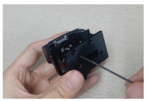
ii. Turn the Cam Pin with flat - headed screwdriver to adjust the blade's height.
