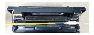
iii. After settling the fiber, turn on the heater by pressing .. (Heating time 20sec)
