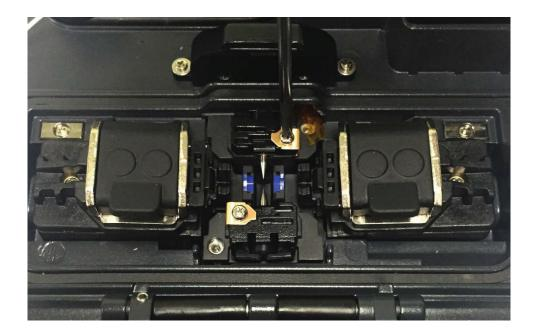
iii. Remove the electrodes block and the electrodes.
